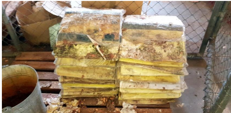
Picture 13: Damage to forms due to water ingress
